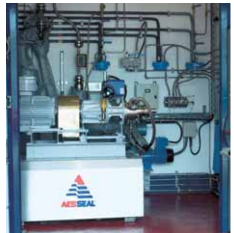
Advanced seal testing on an API 682 specification test rig.
