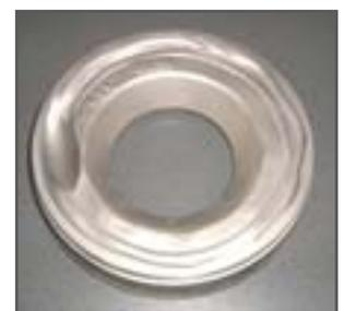
Effects of abrasion and erosion on a seal gland plate.
