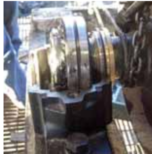
Pulp & Paper Industry, Argentina. 70mm LabTecta-PB™ installed on a SKF® SNL 516-613 pillow block roll (Case Ref: 3217)
