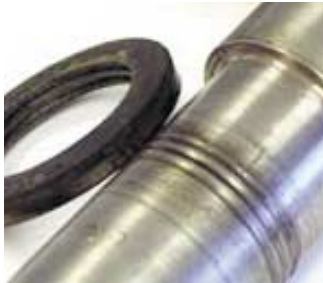
Shaft Damage from a Labyrinth Seal
