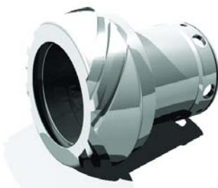
**Figure 5. Using the latest CNC machining techniques, a series of helical vanes are cut in both directions at an approximate angle of 45-deg. The ring is given a shallow tapered contour and operates in a taper-bored cavity.**
