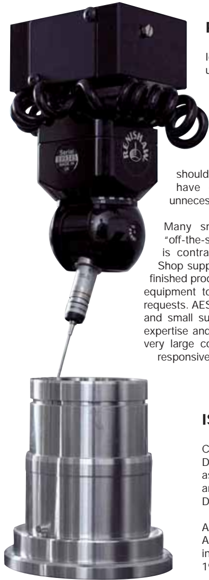
CNC controlled inspection of a seal component.
