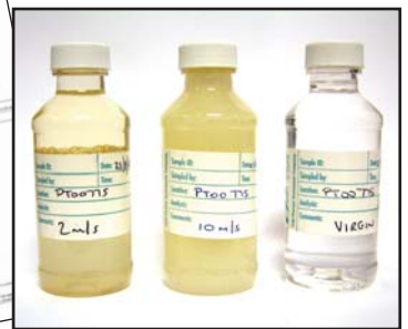
Lip Seal test: Oil sample bottles for laboratory analysis.
